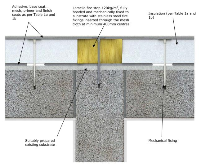
Figure 4: Fire Break Detail
