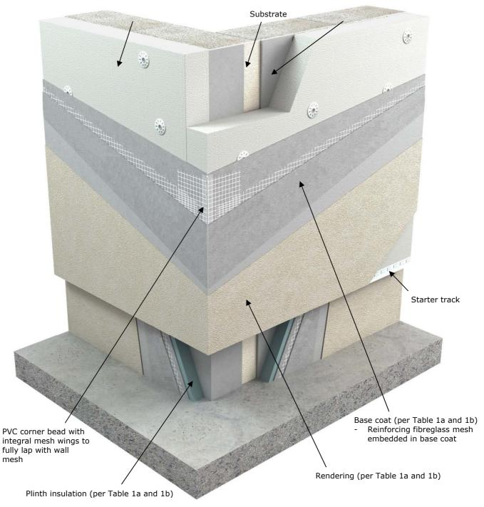
Figure 1: Build-up of System Components
