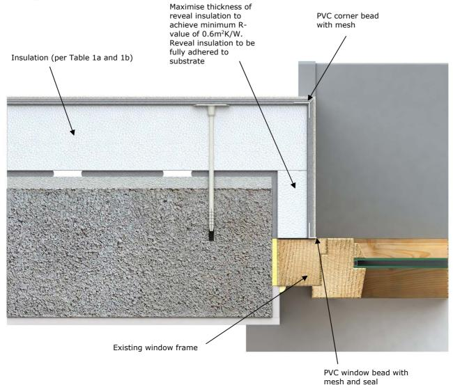
Figure 3: Window Reveal Detail
