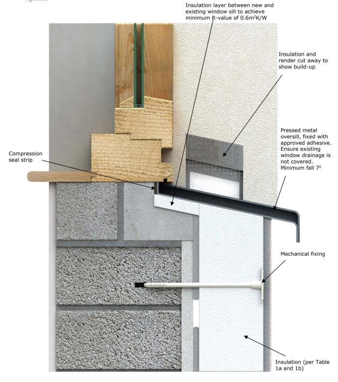
Figure 2: Window Sill Detail
